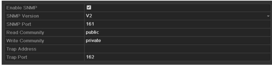
Figure 12-9 SNMP Settings Interface
