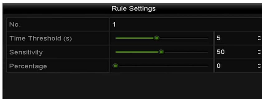
Figure 10-7 Set Intrusion Crossing Detection Rules
