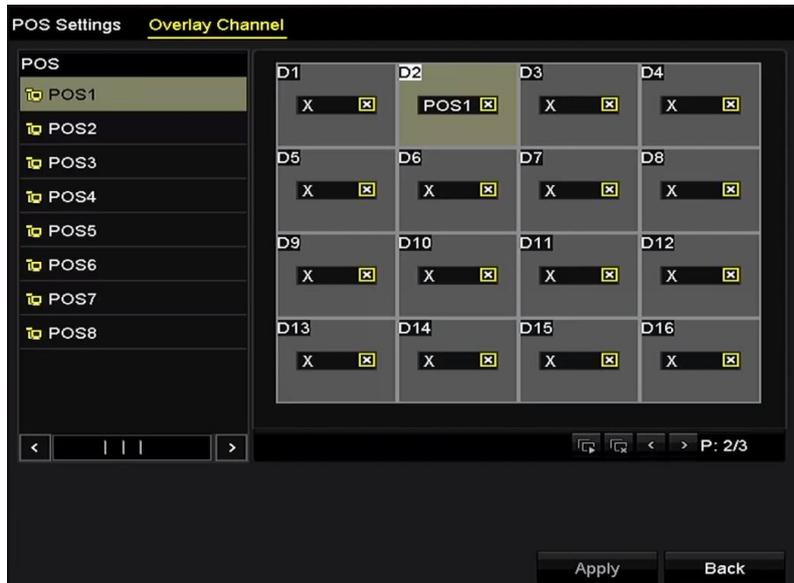
Figure 9-13 Overlay Channel Settings
