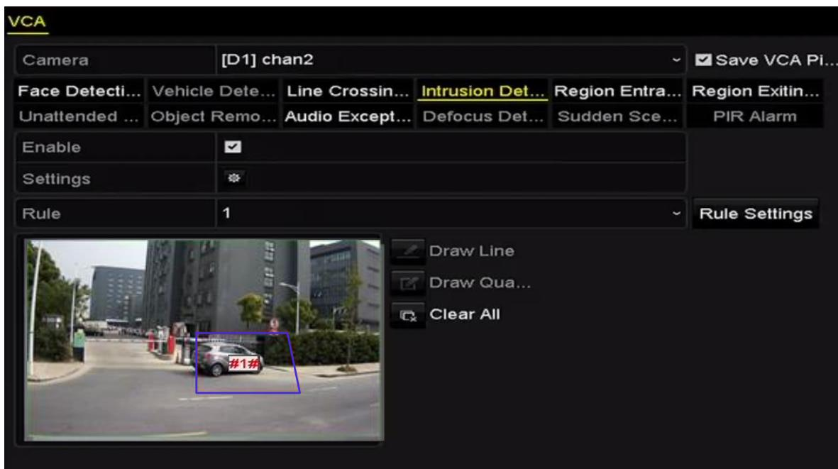
Figure 10-8 Draw Area for Intrusion Detection
