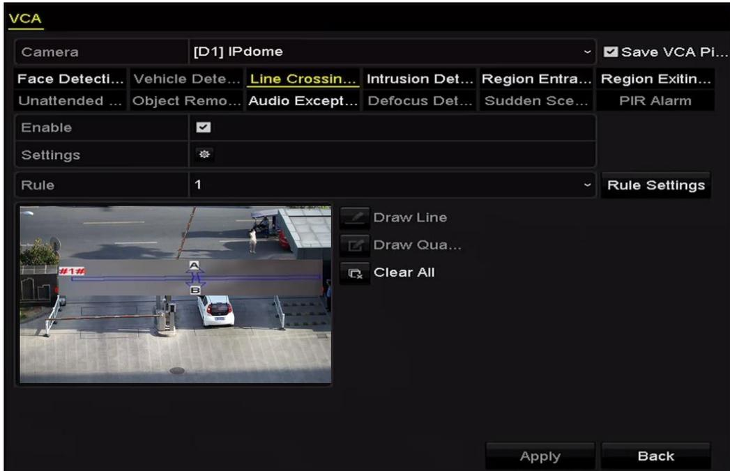
Figure 10-6 Draw Line for Line Crossing Detection
